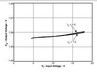
Figure 9. 1.05-V Output Voltage vs Input Voltage
