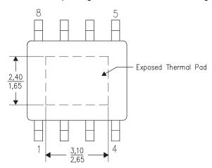
Figure 18. Thermal Pad Dimensions (Top View)
